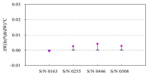
Fig. 5. W(In) changes before and after 1,000 hours exposure at 665°C
