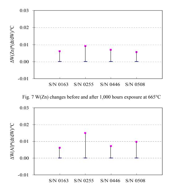
Fig. 8 W(Al) changes before and after 1,000 hours exposure at 665°C
