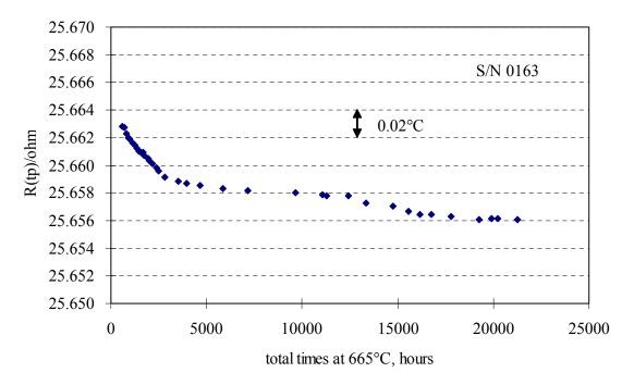
Fig. 1. Long-term stability for a 25-ohm PRT at the triple point of water
