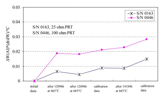
Fig. 3. Long-term stability at the freezing point of aluminum
