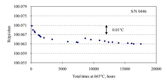
Fig. 2. Long-term stability for a 100-ohm PRT at the triple point of water
